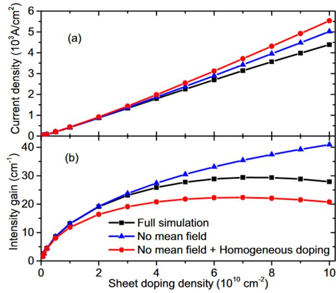
**Fig. 1:** (a) Current density and (b) intensity gain as the function of the sheet doping density for a THz GaAs/AlGaAs QCL (see [3]). The full calculations are indicated by black squares, calculations without considering mean field by blue triangles, and calculations without mean field and assuming a homogeneous doping density by red circles.
