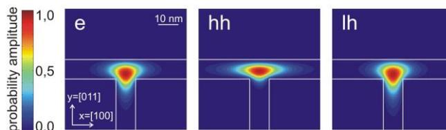
In this figure the calculated wave functions of the electron (e), heavy hole (hh) and light hole (lh) are shown.
