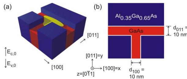
The figure on the left (a) shows schematically the conduction band profile of a T-shaped quantum wire. The schematic on the right (b) shows the relevant dimensions and materials.
