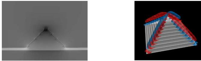
Left: Cut through the quantum dot: The bright line represents a layer of three atomic layers of InAs. Below this InAs layer the substrate material GaAs is located. The different lattice constants of GaAs and InAs lead to strain which causes self-organized growth of quantum dots. The InAs pyramid is surrounded by GaAs.
