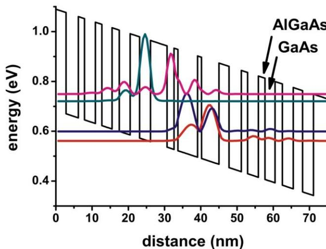
Conduction band structure of a quantum cascade laser including the most important electron wave functions.
